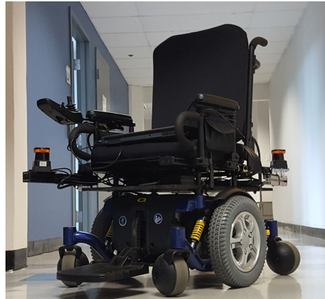
Figure 1: The Vulcan Intelligent Wheelchair: one of the robot platforms used in the presented work.
